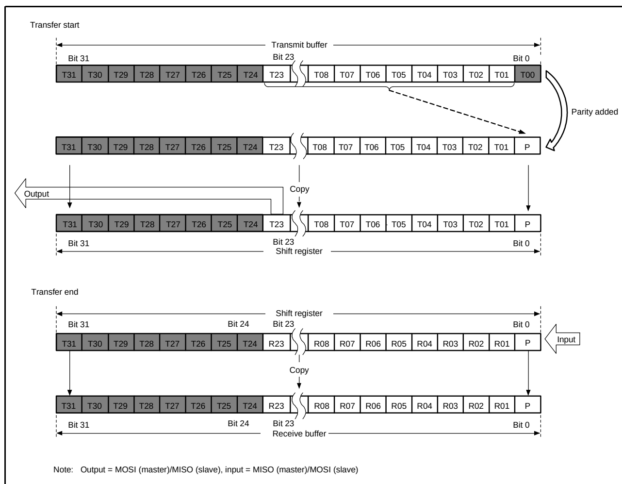
Figure 27.19 MSB First Transfer (24-Bit Data, Parity Enabled)
