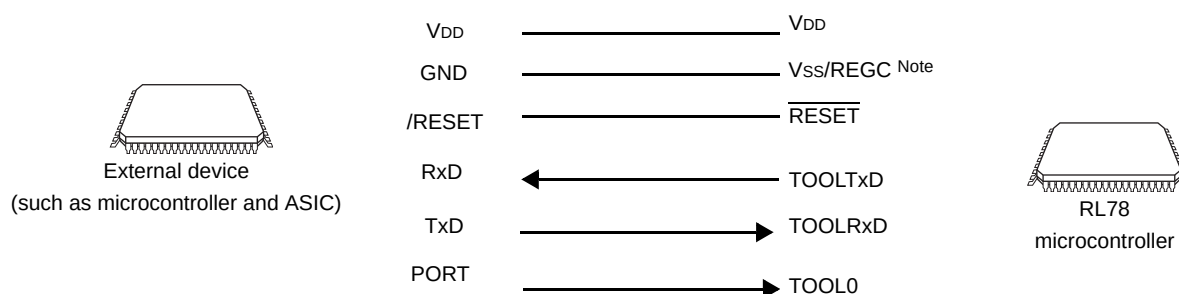
Figure 36 - 4 Communication with External Device
