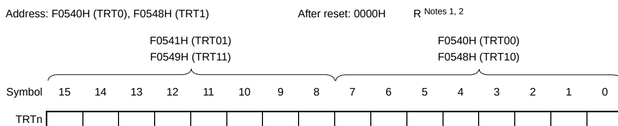
Figure 12 - 3 Format of 8-bit interval timer counter register n (TRTn)
