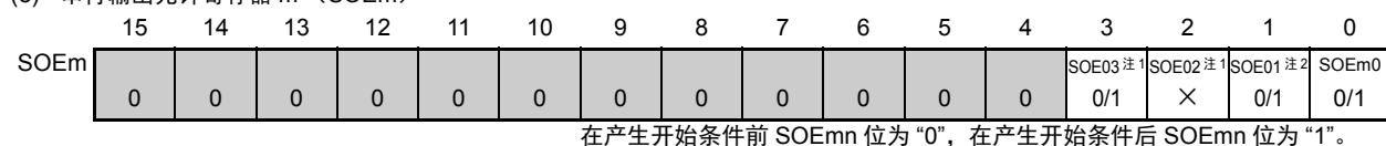
(e) 串行输出允许寄存器 m (SOEm m )
